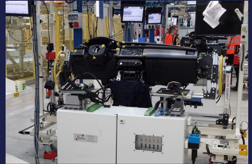
Automotive cockpit end of line test system
